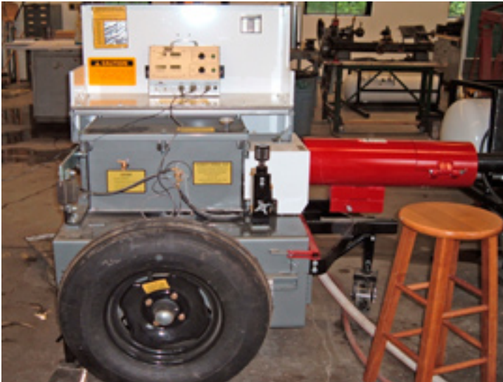
FIGURE 4. AW Dynamometer Model NEB460 dynamometer used to measure torque.
